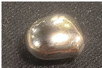
Vacuum arc melt SMA buttons
