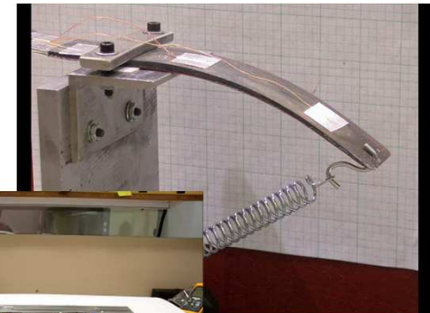
Hinge Line Integrated SMA Tube
