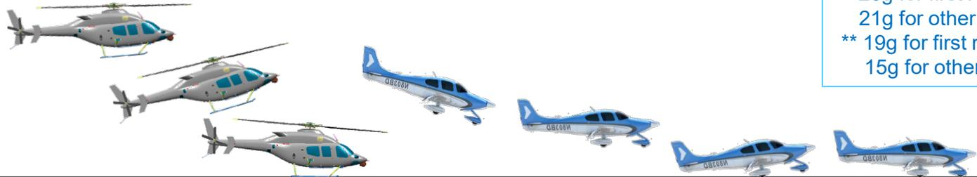
Statistical data used to establish emergency landing conditions for rotorcraft § 27.562(b) and general aviation airplanes § 23.562(b) reveal they crash at about the same impact velocities but different decelerations
