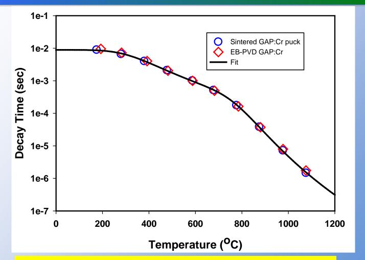
Decay time  $(\tau_2)$  vs. temperature dependence for thin EB-PVD Cr:GAP coating follows same calibration curve as Cr:GAP puck.
