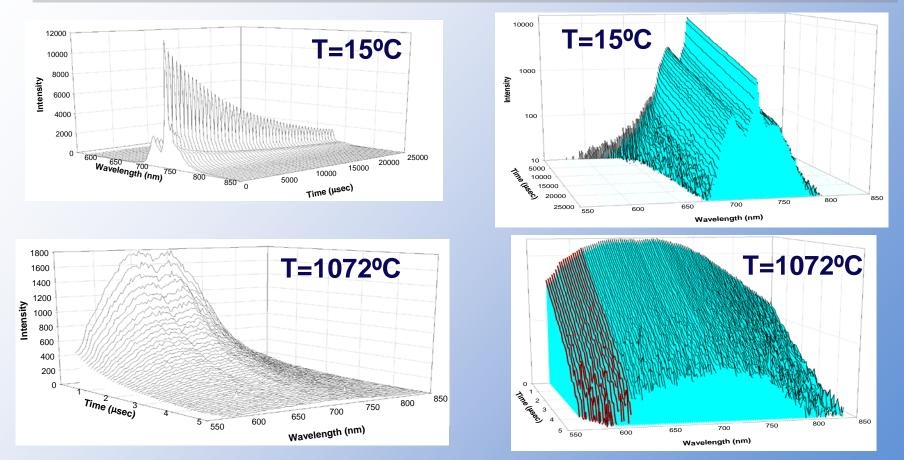
Logarithmic intensity scale shows uniform decay rate over full wavelength range at each T.
