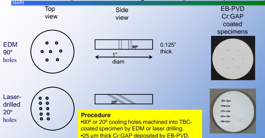
Specimens ready for 2D mapping of thermal gradients around cooling holes during exposure to high heat flux laser. Scheduled for July 2012 for completion of Phase I milestones.
