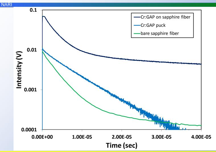
•Intrinsic luminescence from sapphire fiber overwhelms Cr:GAP luminescence.
