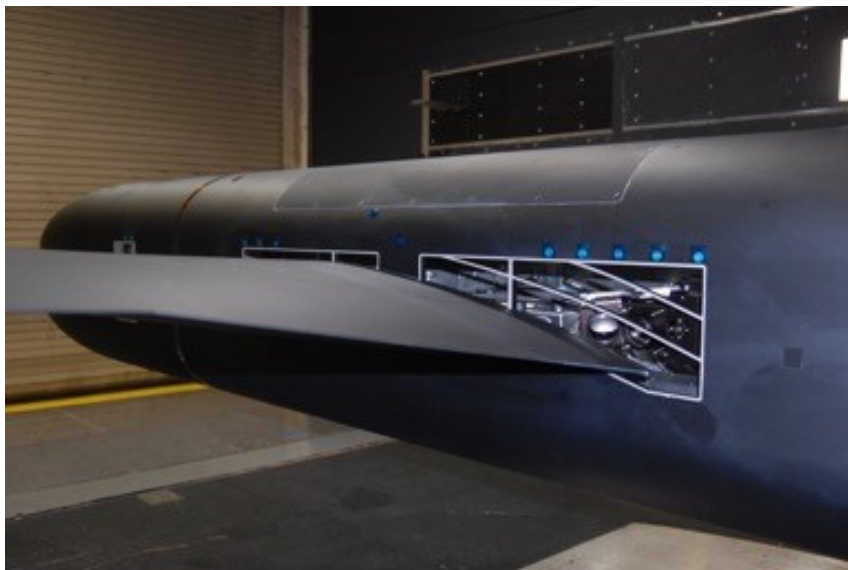
NASA Juncture Flow Experiment in LaRC 14'x22' wind tunnel
