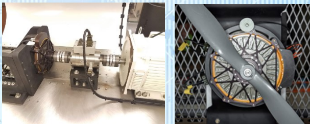
Baseline Motor Testing for baseline performance
