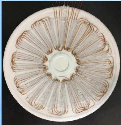
Demonstrations were made with 30 AWG Kapton™ coated litz wire on polycarbonate
