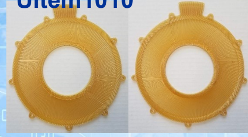
Concept B - Stator Plates from Ultem1010
