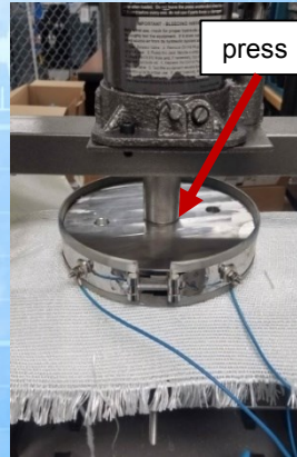
Pressing process needed to further densify the stator
