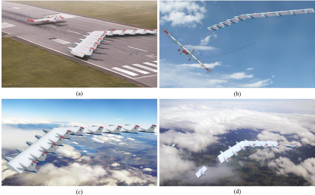
**Figure 2. Conceptual image of the Cluster Wing vehicles (a) Takeoff with tow aircraft (b) Tow aircraft releases the Cluster Wing at top of climb (c) Vehicles together during cruise (d) Vehicles separating to complete mission**
