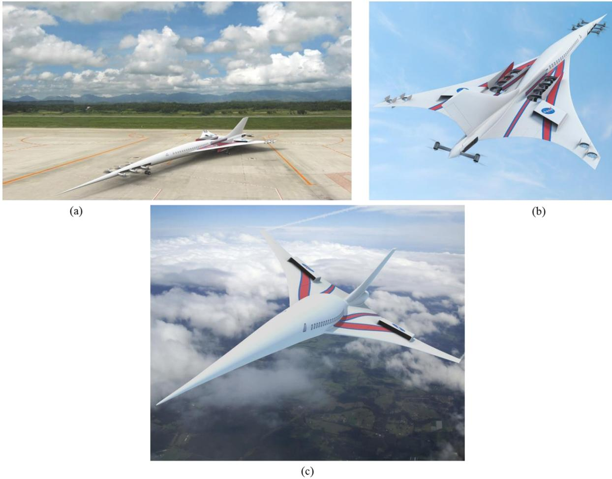
**Figure 3. Supersonic VTOL concept aircraft (a) With rotors deployed for vertical takeoff (b) In transition flight from vertical takeoff to horizontal flight (c) With rotors retracted during cruise flight**
