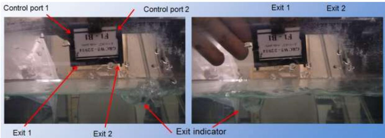
**Figure 16. Functioning of a fluidic diverter.**
