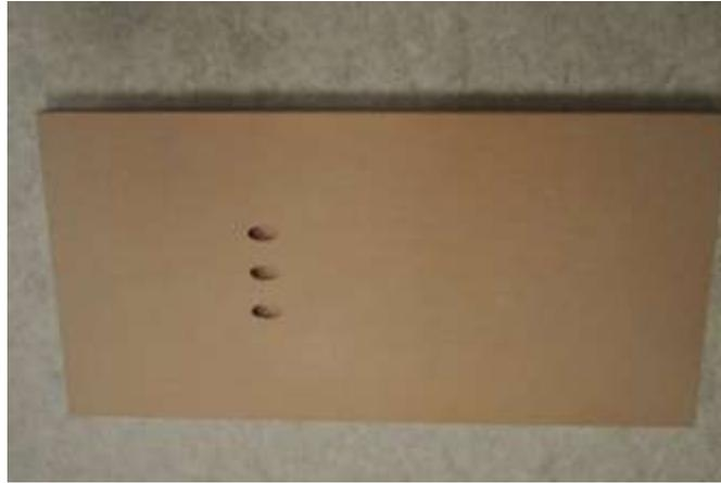
Figure 9. Alumina coupon to be tested in burner rig.
