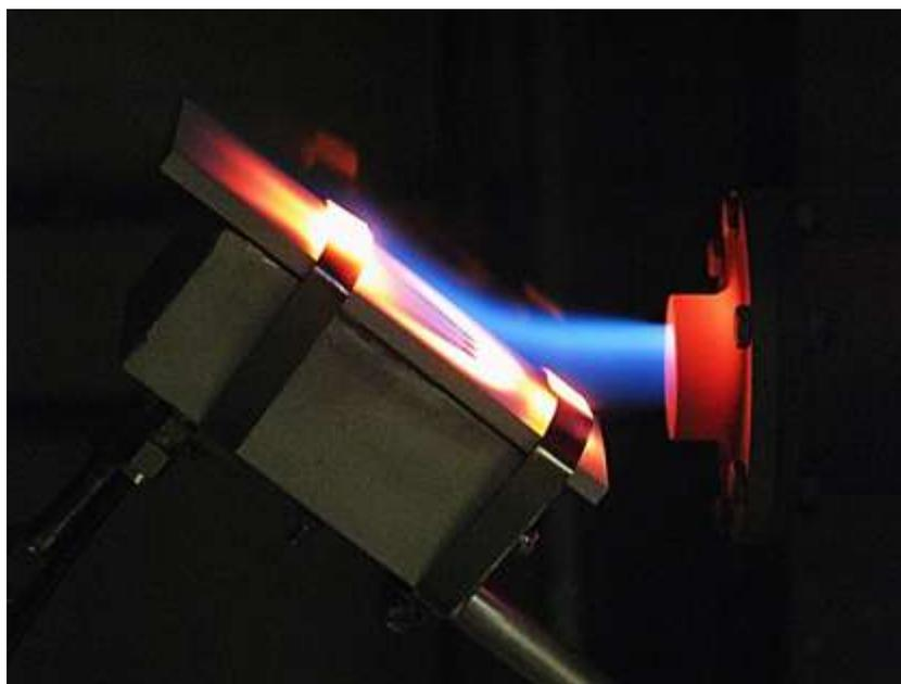
Figure 6. Mach 0.3 burner jet impinging on a coupon.
