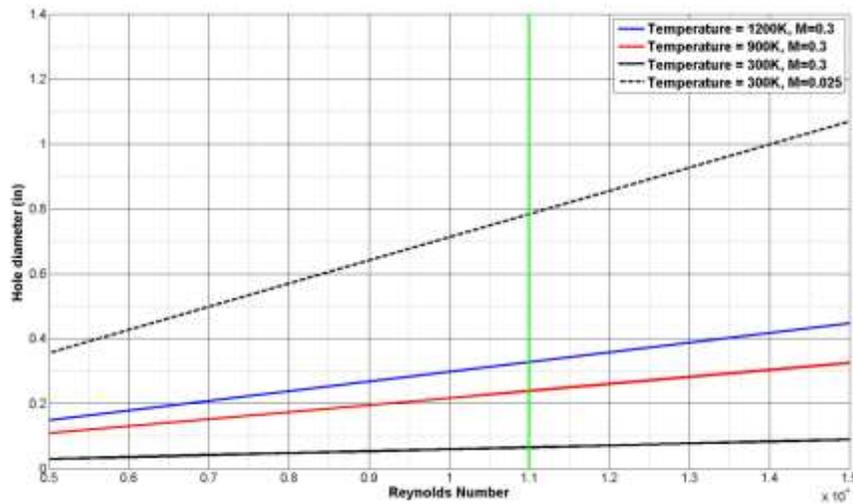
Figure 112. Scaling cooling holes with temperature and Mach number.
