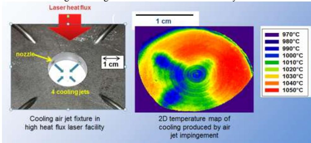
Figure 8. effect of cooling air jet impingement on a laser-heated button specimen
