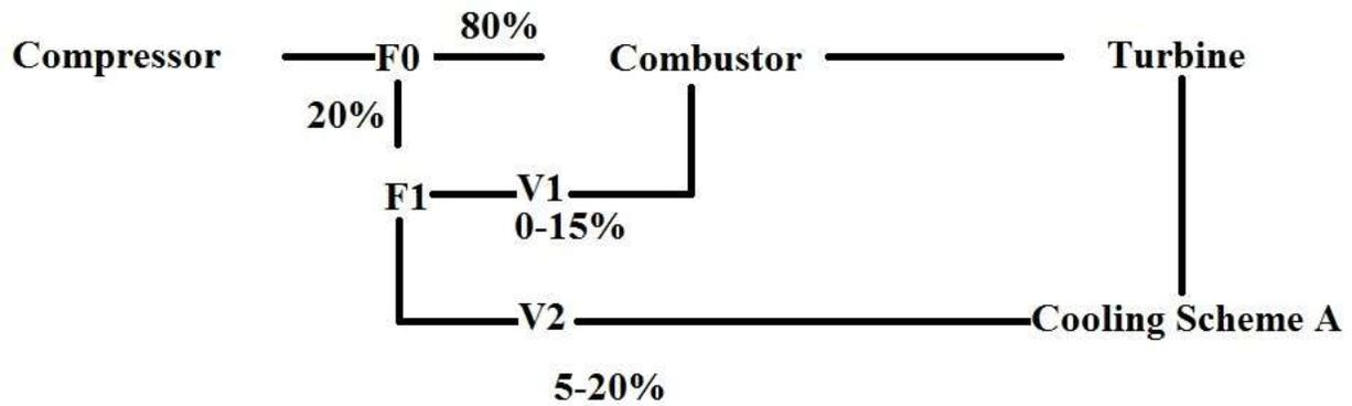
Figure 19. Flowchart of cooling scheme with modulation.
