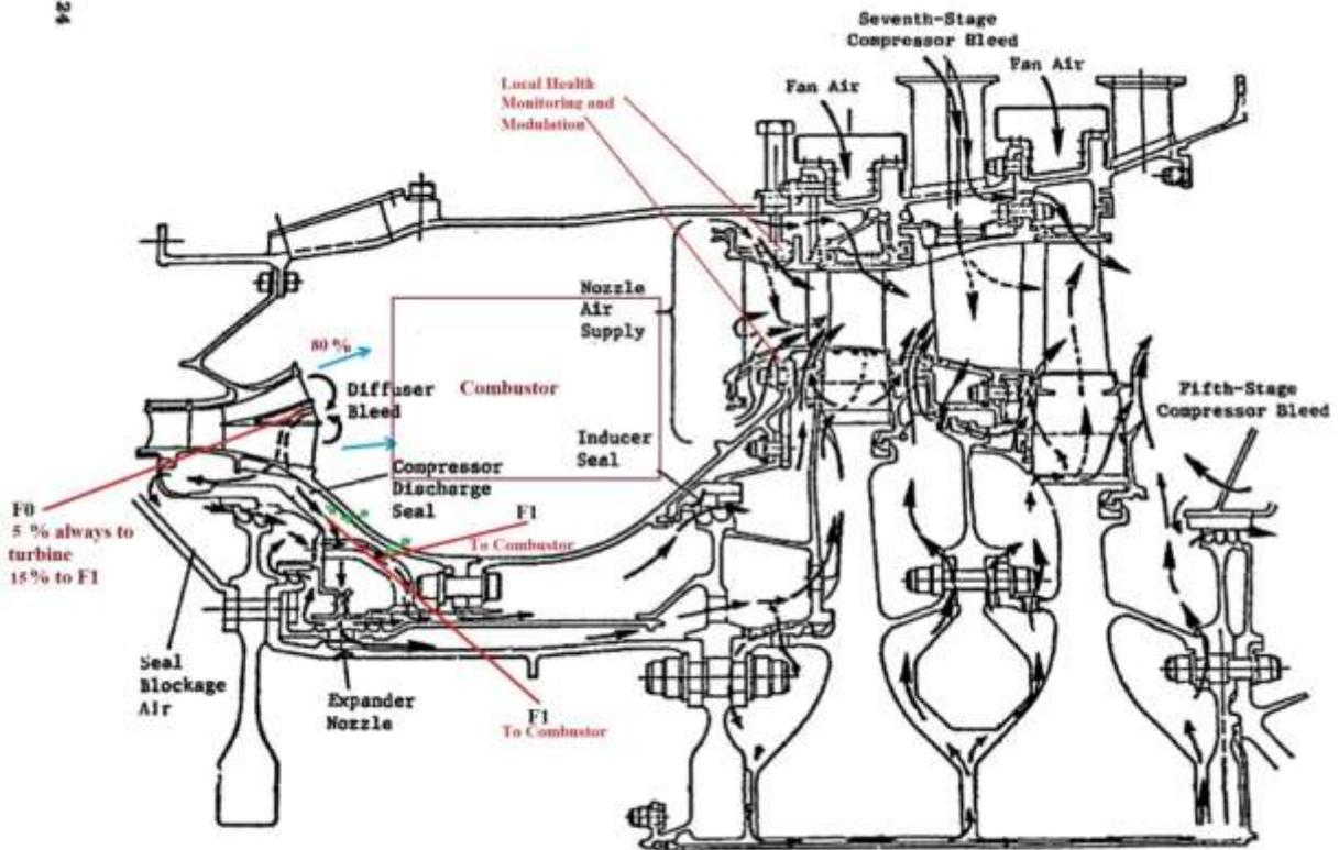
Figure 11. Rotor and Casing Cooling-Supply System.
