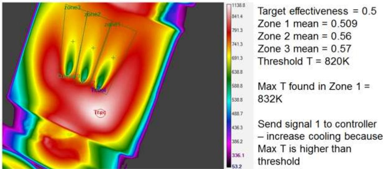
Figure 23. Example 3 of thermal map for modulation control.
