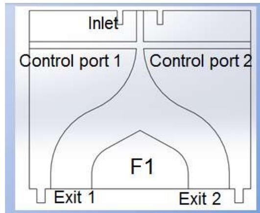
Figure 14. Example of a fluidic diverter, F1.
