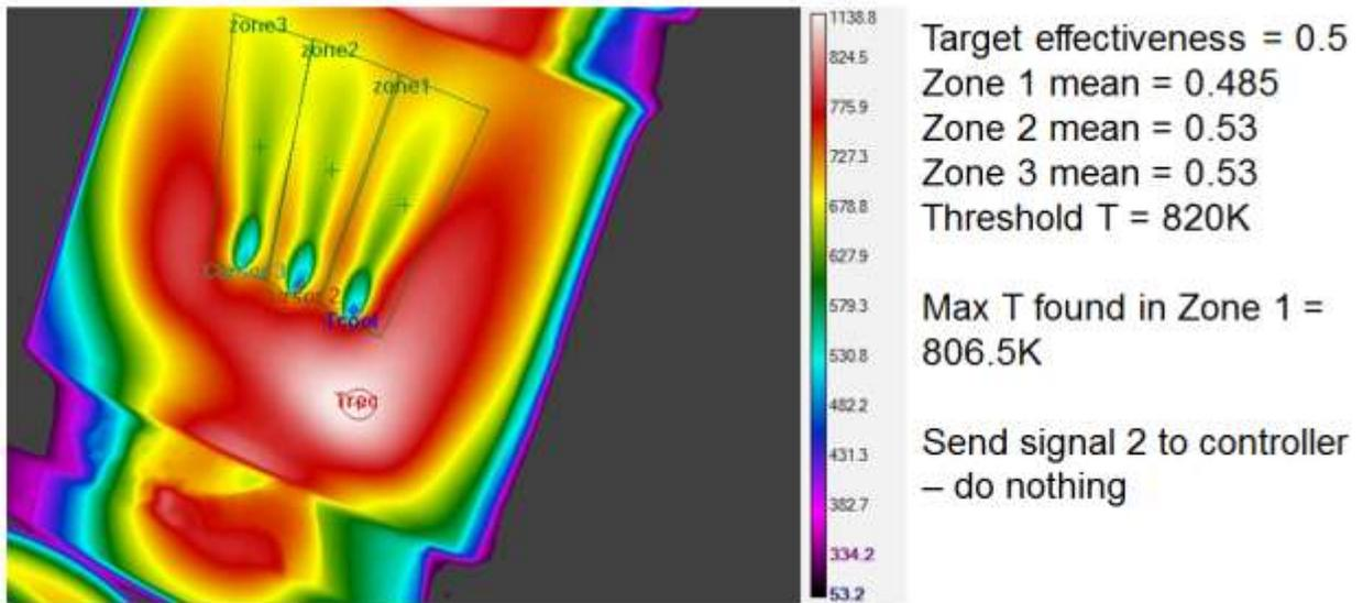
Figure 13. Example 2 of thermal map for modulation control.
