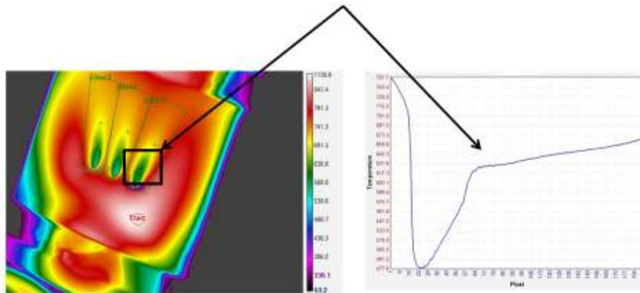
Figure 24. Sample temperature profile downstream of high blowing ratio cooling jet.
