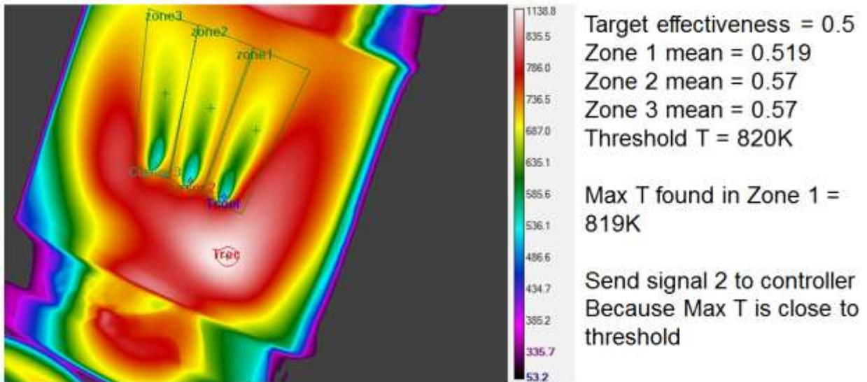
Figure 21. Example 1 of thermal map for modulation control.
