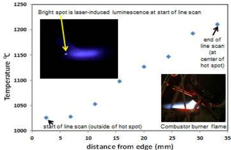
**Figure 1. Luminescence based temperature measurements.**
