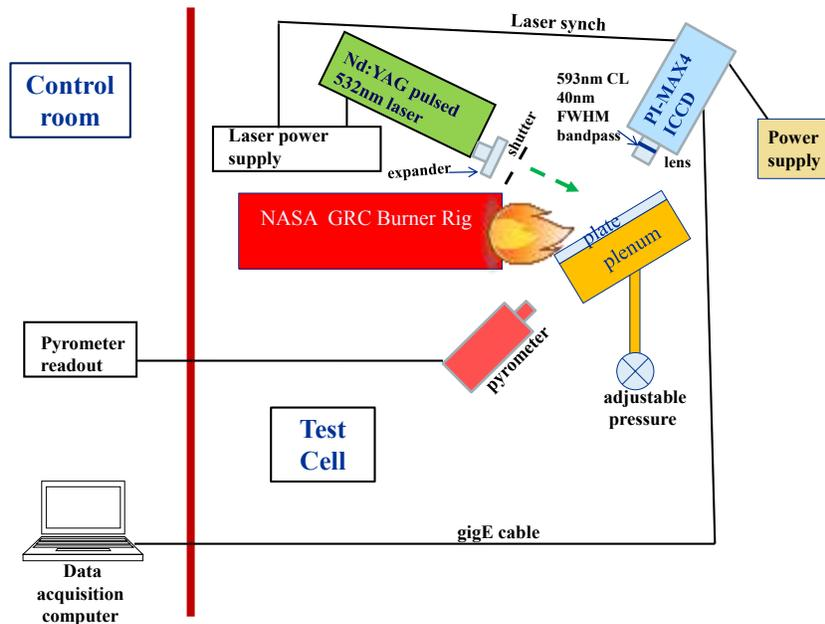
Figure 7. Schematic of luminescence based temperature measurement experiment.
