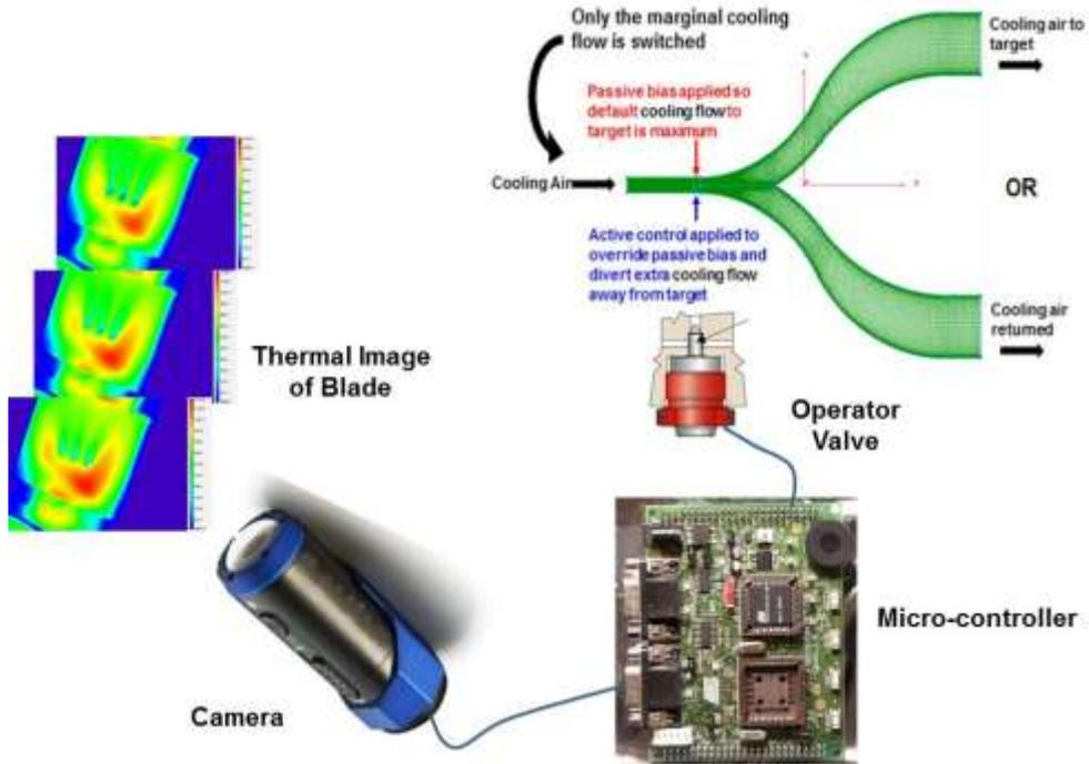
Figure 17. Schematic of modulation system.
