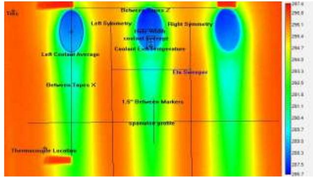
Figure 101. Infrared image of film-cooled flat plate
