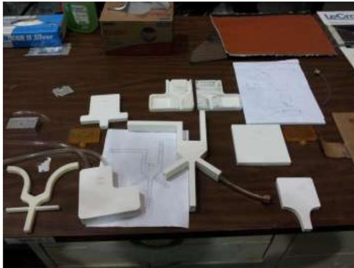
**Figure 125. Fluidic devices tested using additive manufacturing.**
