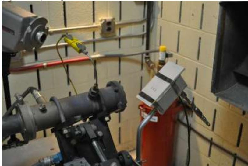
Figure 5. Setup of coupons for infrared thermography in Mach 0.3 burner rig.
