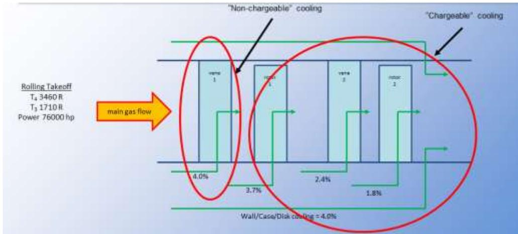
Figure 3. Cooling flow breakdown for N+2 turbofan with cooled, two-stage high pressure turbine
