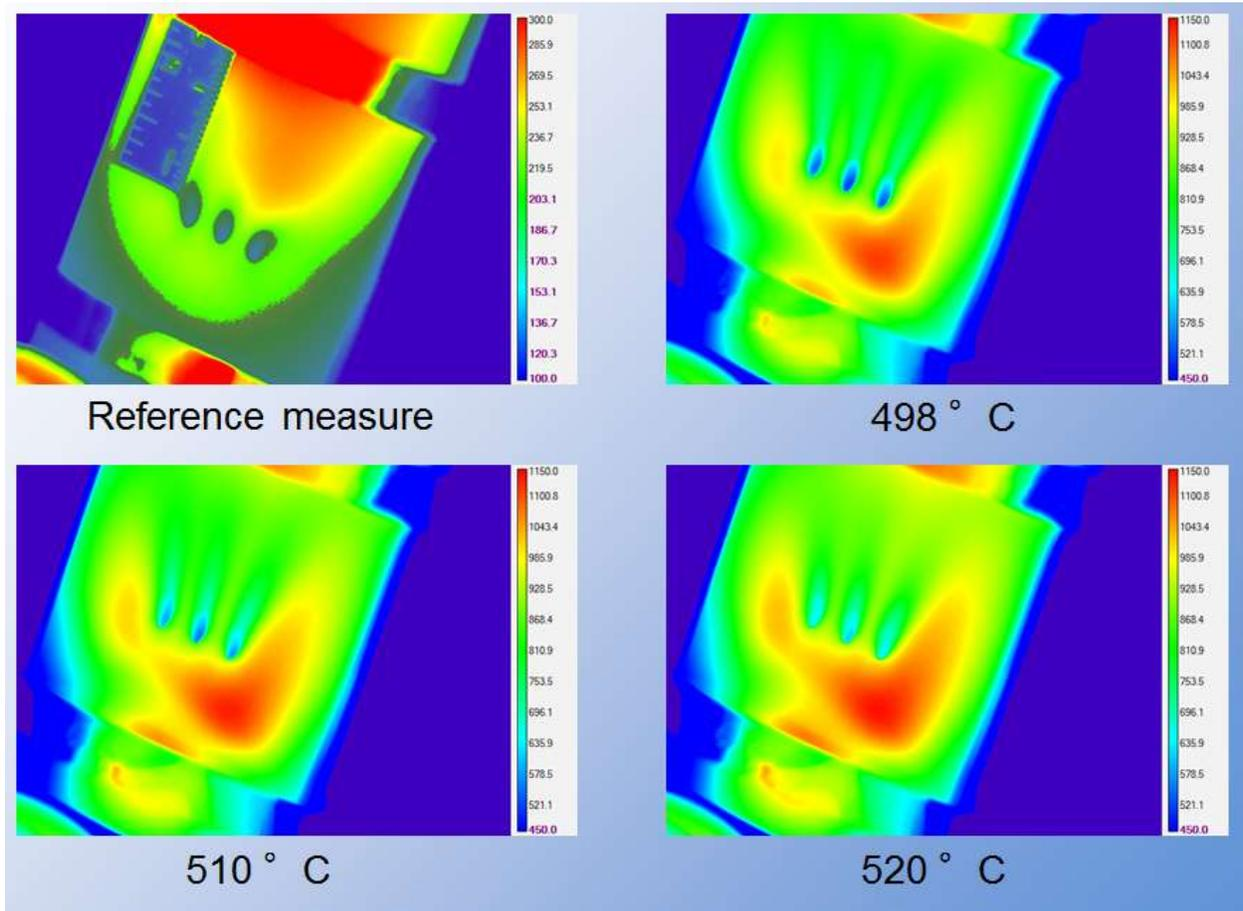
Figure 13. Film cooling coupon at different temperatures to show differing thermal patterns on surface.
