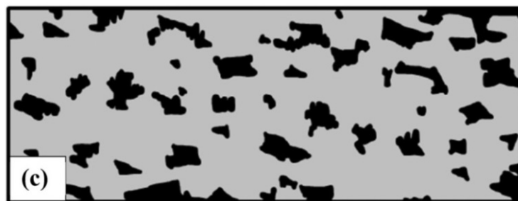
Figure 27.—(a) Optical view of the top surface of a Sylramic preform; (b) CT scan of the cross-section of the preform; and (c) schematic of the cross-section showing the distribution of voids. The area fraction of the voids was estimated by image analysis of the CT scan was 21 to 23%.
