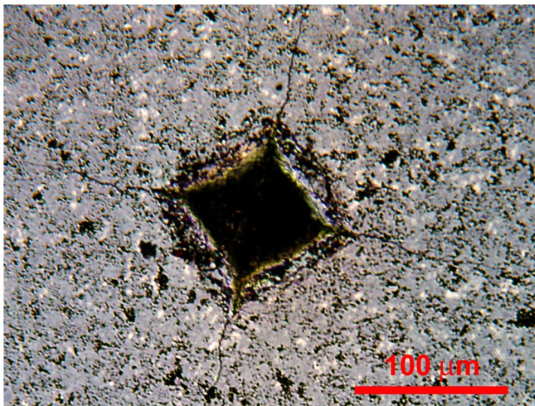
Figure 9.—Photograph of a Vickers hardness indent showing cracks (red arrows) emanating from it. These specimens will be oxidized at high temperatures to study the effect of additives on the self-healing of these cracks.
