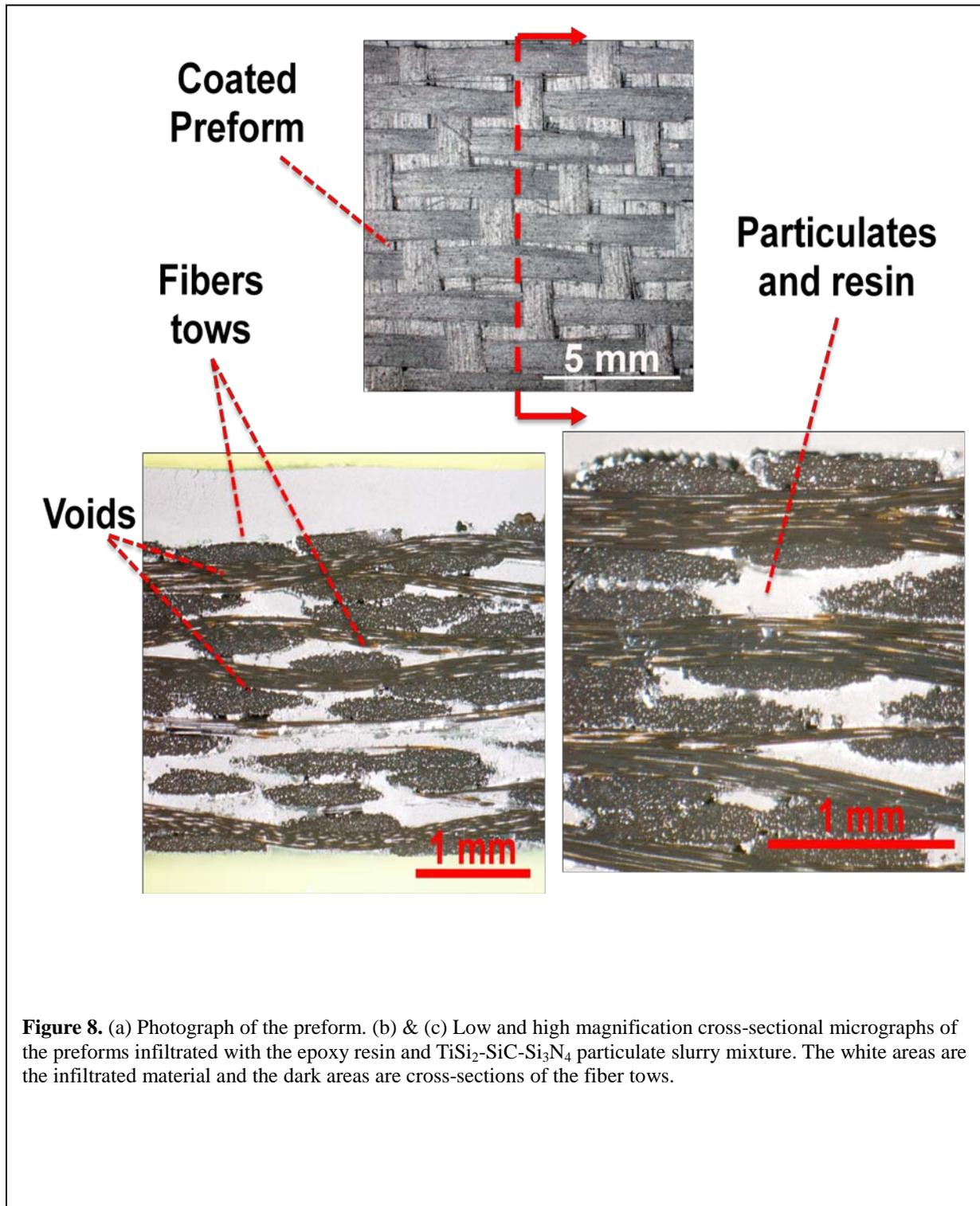
**Figure 8.** (a) Photograph of the preform. (b) & (c) Low and high magnification cross-sectional micrographs of the preforms infiltrated with the epoxy resin and  $\text{TiSi}_2\text{-SiC-Si}_3\text{N}_4$  particulate slurry mixture. The white areas are the infiltrated material and the dark areas are cross-sections of the fiber tows.
