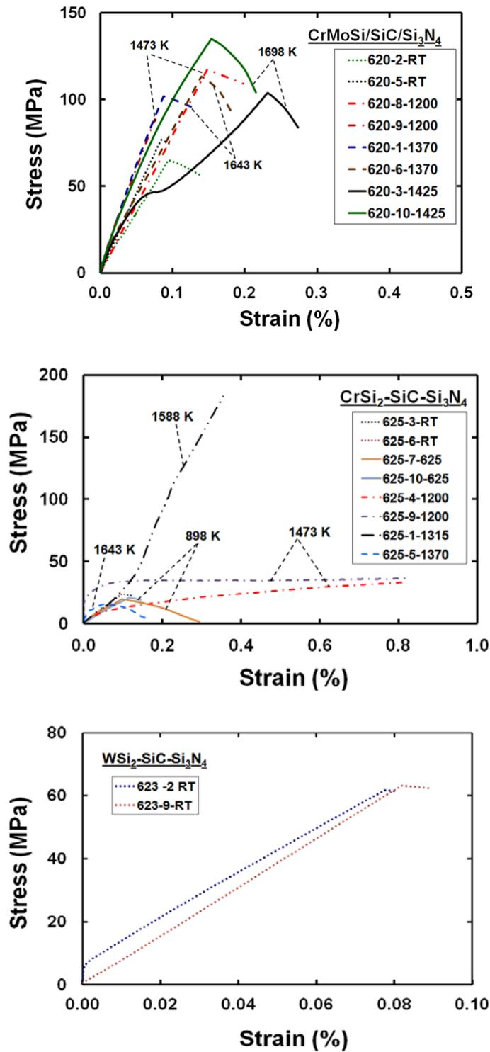
**Figure 7.** Bend stress-strain data for CrMoSi-SiC-Si<sub>3</sub>N<sub>4</sub>, CrSi<sub>2</sub>-SiC-Si<sub>3</sub>N<sub>4</sub> and WSi<sub>2</sub>-SiC-Si<sub>3</sub>N<sub>4</sub> specimens tested at room temperature, 1473, 1643 and 1698 K. The WSi<sub>2</sub>-SiC-Si<sub>3</sub>N<sub>4</sub> underwent catastrophic oxidation during heat-up to high temperatures.
