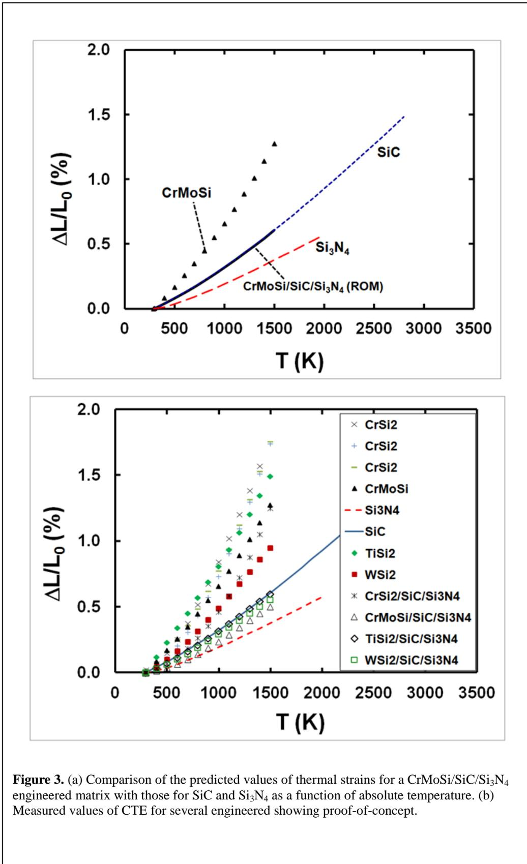
**Figure 3.** (a) Comparison of the predicted values of thermal strains for a CrMoSi/SiC/Si<sub>3</sub>N<sub>4</sub> engineered matrix with those for SiC and Si<sub>3</sub>N<sub>4</sub> as a function of absolute temperature. (b) Measured values of CTE for several engineered showing proof-of-concept.
