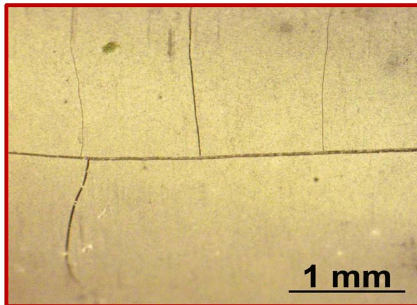
**Figure 5.** Macrograph of the surface of a  $\text{MoSi}_2/\text{SiC}/\text{Si}_3\text{N}_4$  CTE specimen showing extensive cracks after three thermal cycles.
