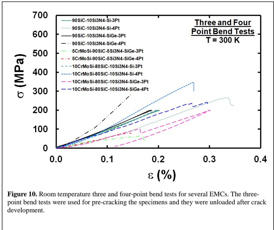
**Figure 10.** Room temperature three and four-point bend tests for several EMCs. The three-point bend tests were used for pre-cracking the specimens and they were unloaded after crack development.
