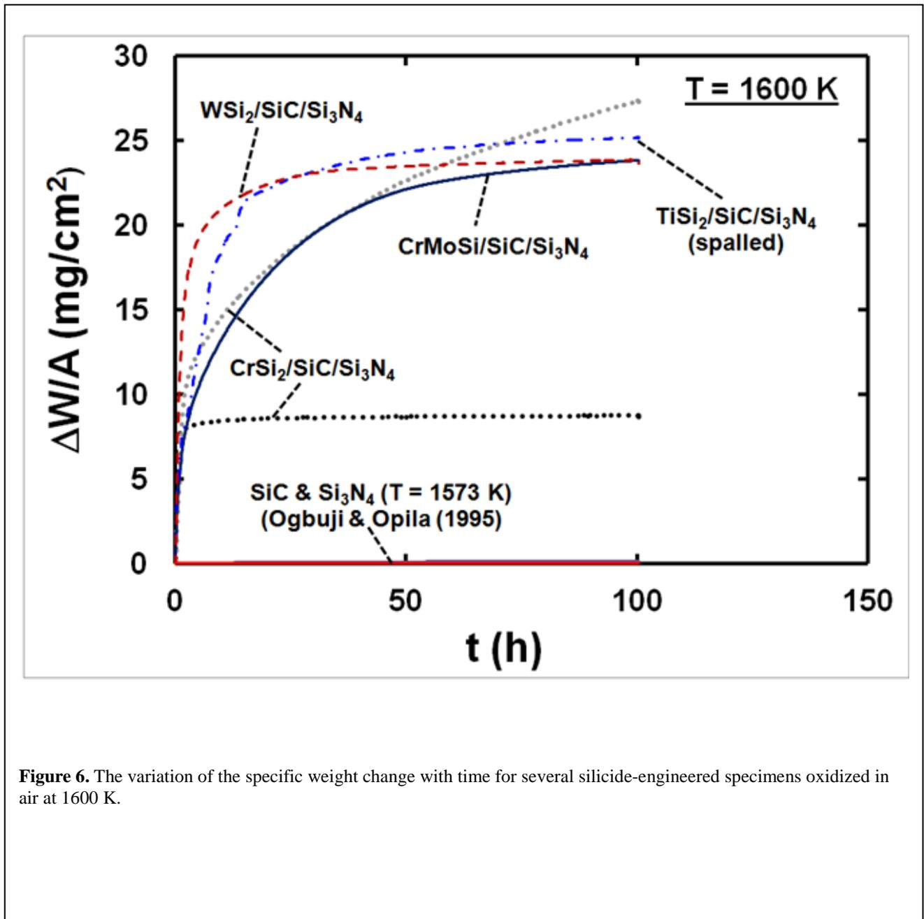
**Figure 6.** The variation of the specific weight change with time for several silicide-engineered specimens oxidized in air at 1600 K.
