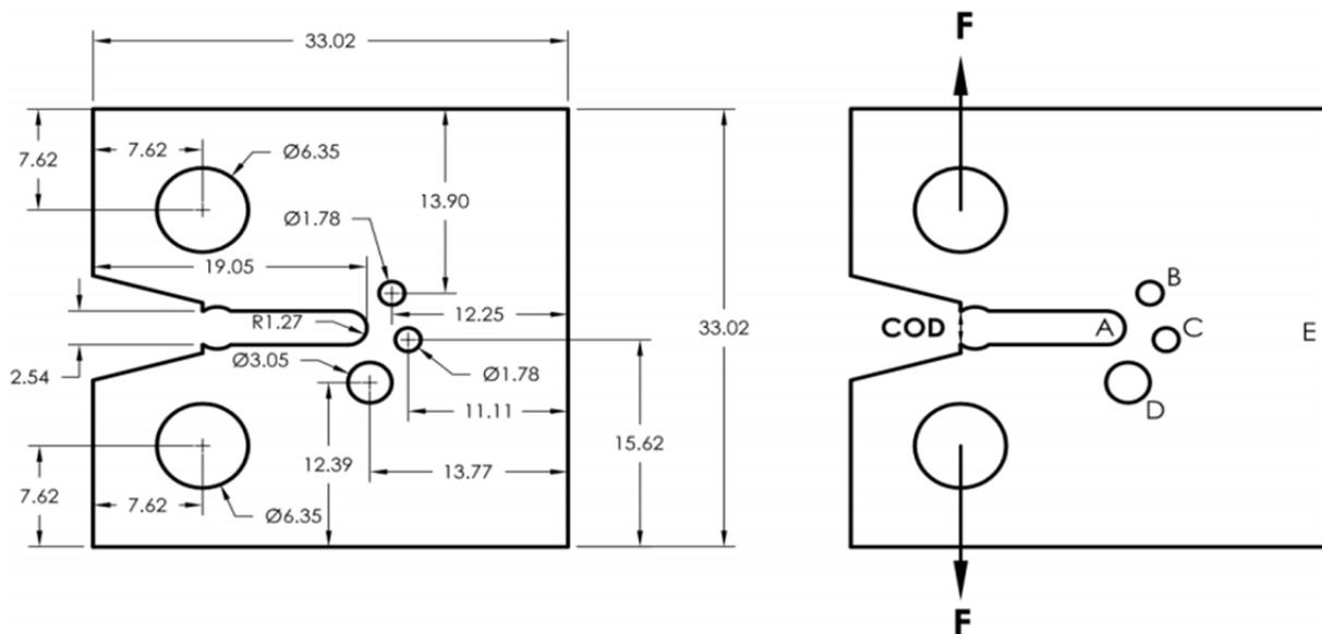
Figure 2: Challenge specimen configuration, thickness = 3.18 mm (to scale) [8].
