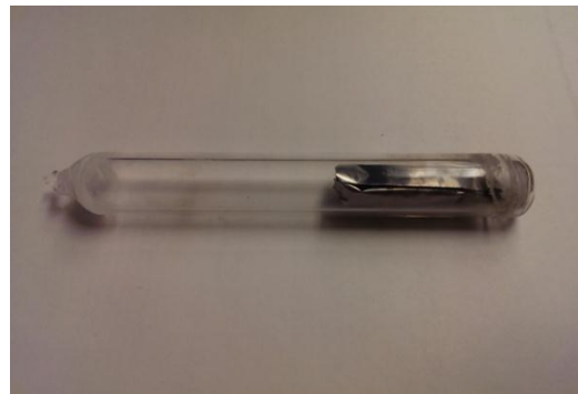
Figure 5 Sealed quartz tube containing cold a pressed alloy pellet ready for sintering.
