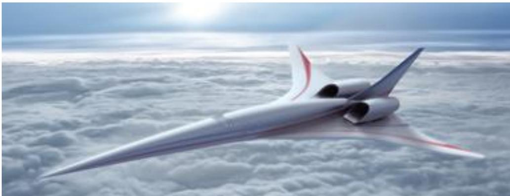
**Figure 8: NASA Low Boom Supersonic Transport Concept.**
