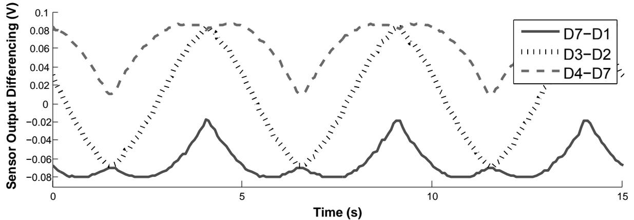
Fig. 13. Sensor output differencing based on a 5 mm target moving 1.47 cm across the sensor FOV at 0.2 Hz.
