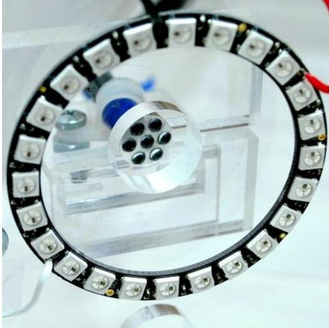
**Fig. 9. Close up of the sensor head and LED array on the mount.**
