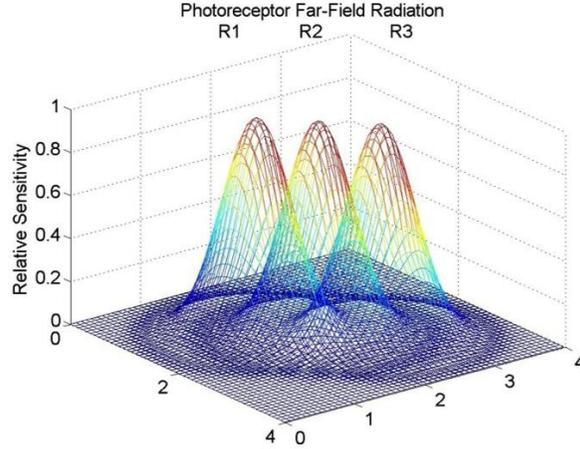
**Fig. 1. Depiction of overlapping Gaussian response observed by the compound eye sensor**
