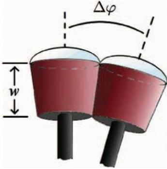
**Fig. 3. Detail of two photoreceptors in sensor head, where  $w$  represents the distance between the lens and the image plane and  $\Delta \phi$  represents the angle between two lenses.**
