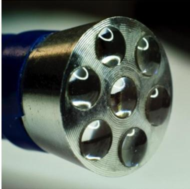
**Fig. 2. Front view of sensor head or “photoreceptor”.**
