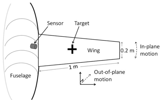
**Fig. 11. Sensor-target arrangement on an aircraft.**
