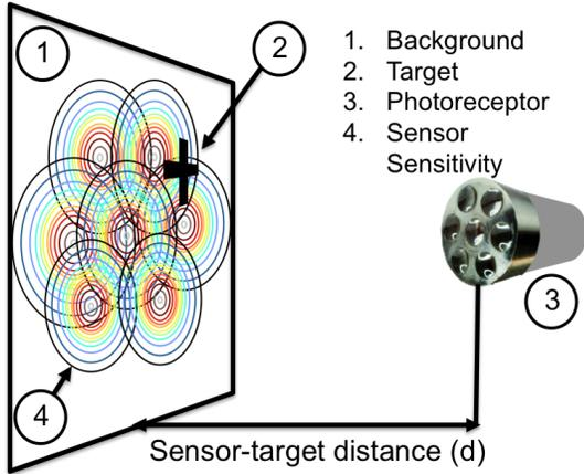
Fig. 4. Simulation experimental setup.
