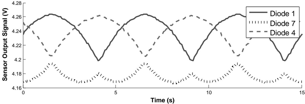
**Fig. 12. Sensor output based on a 5 mm target moving 1.47 cm across the sensor FOV at 0.2 Hz.**
