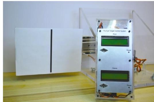
**Fig. 10. The target position control system and remote controller.**
