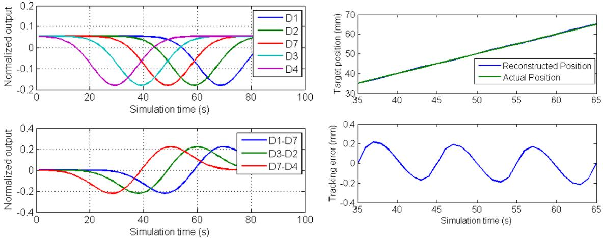
**Figure 7. Simulation signals (top), difference signals (e.g., diode D1 – diode D7) (bottom).**
