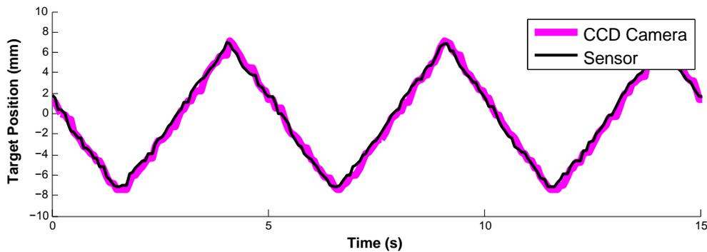
Fig. 14. Target position with time as determined by sensor and CCD camera tracking algorithms.
