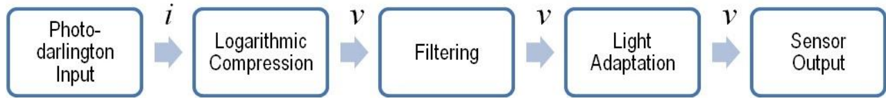
Fig. 4. Block diagram of sensor functionality through a single channel, where i represents current and v represents voltage.
