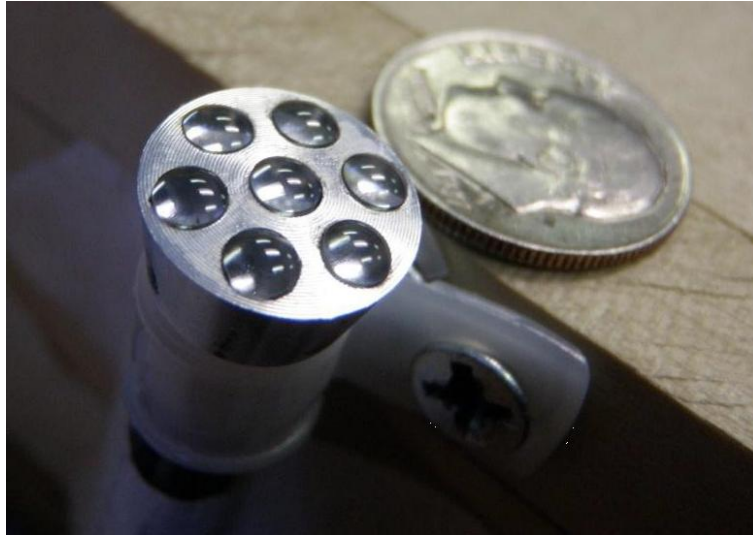
Fig. 5. Front view of sensor head with U.S. dime for comparison.
