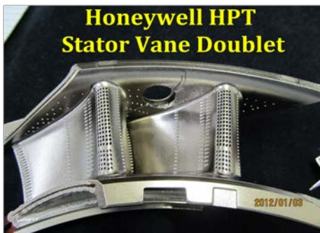
Figure 17. Honeywell stator vane doublet selected for 2D temperature mapping around cooling holes in combustion environment for Phase II.
