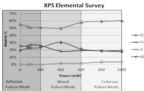
**Figure 4.** XPS survey scan data showing the atomic percent abundance of select elements found in survey scan spectra. Shading on the figure indicates the dominant failure mode seen in SLS test specimens.
