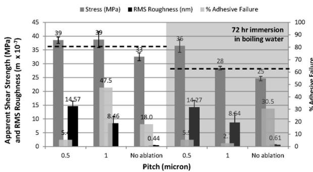
**Figure 7. Results for PETI-5 SLS specimens prepared with polished adherends. Laser power was 1 W for all ablated specimens. Data in the shaded region was collected from specimens that underwent a 72 h immersion in boiling water immediately prior to testing. Dashed lines indicate the apparent shear strength values achieved for unpolished SLS specimens. ( $1 \times 10^{-7} \text{ m} = 0.1 \mu\text{m}$ ).**
