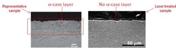
**Figure 2. SEM images showing  $\alpha$ -case layer in Ti alloy.**
