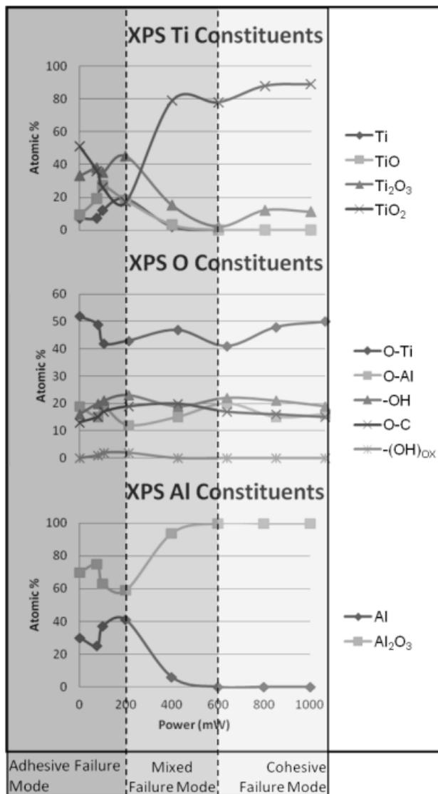
**Figure 6.** Atomic percent abundance of surface constituents based on the deconvolution of the Ti2p<sub>1/2</sub> and Ti2p<sub>3/2</sub> multiplex (top), O1s peak (center), and Al2p peak (bottom). Shading on the figure indicates the dominant failure mode seen in SLS test specimens.
