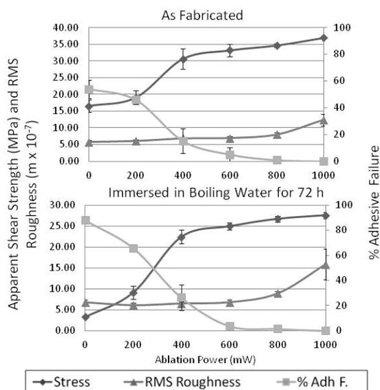
**Figure 9.** Roughness and lap shear data for non-polished, laser ablated adherends are shown for two data sets: laser power variation without (top) and with (bottom) immersion in boiling water. ( $1 \times 10^{-7} \text{ m} = 0.1 \mu\text{m}$ ). Ablation pitch was 25.4  $\mu\text{m}$  for all specimens.
