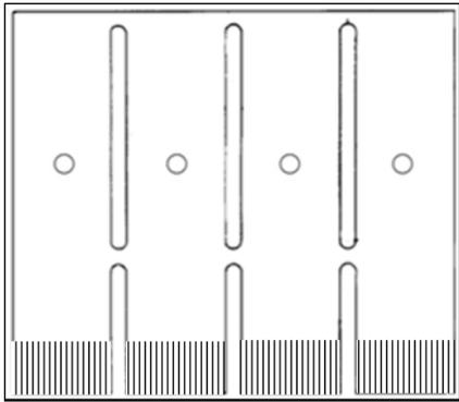
**Figure 11. Modified single-lap shear adherend geometry indicating laser-etched portion.**
