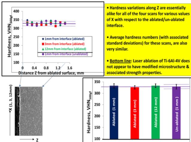
**Figure 3. Microhardness characterization results from a laser ablated Ti-6Al-4V surface.**
