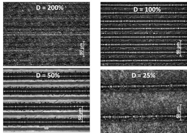
**Figure 1: Parallel lines ablated into a Ti-6Al-4V surface with a pitch of: (upper left) 0.013 mm (0.0005 in), (upper right) 0.025 mm (0.001 in), (lower left) 0.051 mm (0.002 in) and (lower right) 0.102 mm (0.004 in).**
