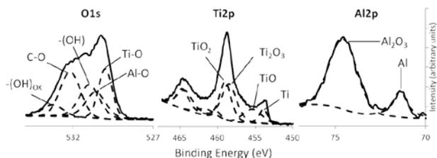
**Figure 5.** De-convolution of a high-resolution O1s, Ti2p, and Al2p spectra from different specimens showing peak assignments.
