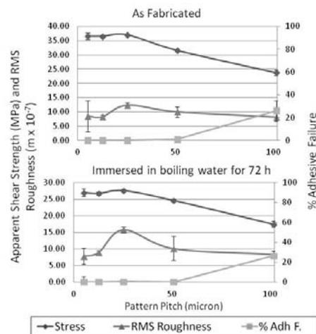
**Figure 8. Apparent shear strength, failure mode and roughness results for non-polished adherends are shown for two data sets: variation of ablation line pitch without (top) and with (bottom) immersion in boiling water. ( $1 \times 10^{-7} \text{ m} = 0.1 \mu\text{m}$ ).**
