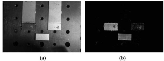
**Figure 12. On the left is a visible light image of a failed lap-shear specimen showing mostly adhesive failure. On the right is a fluorescence image of the same specimen with clearly visible adhesive residues. A 12.7 x 25.4 mm (0.5 in x 1 in) reference standard with a fluorescent coating is visible at the bottom of each image.**
