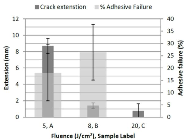
**Figure 10. Crack extension and failure mode data for wedge test specimens ablated with three different laser fluence levels.**
