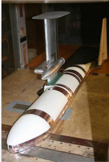
Figure 20 PTERA C-3 Wind tunnel model
