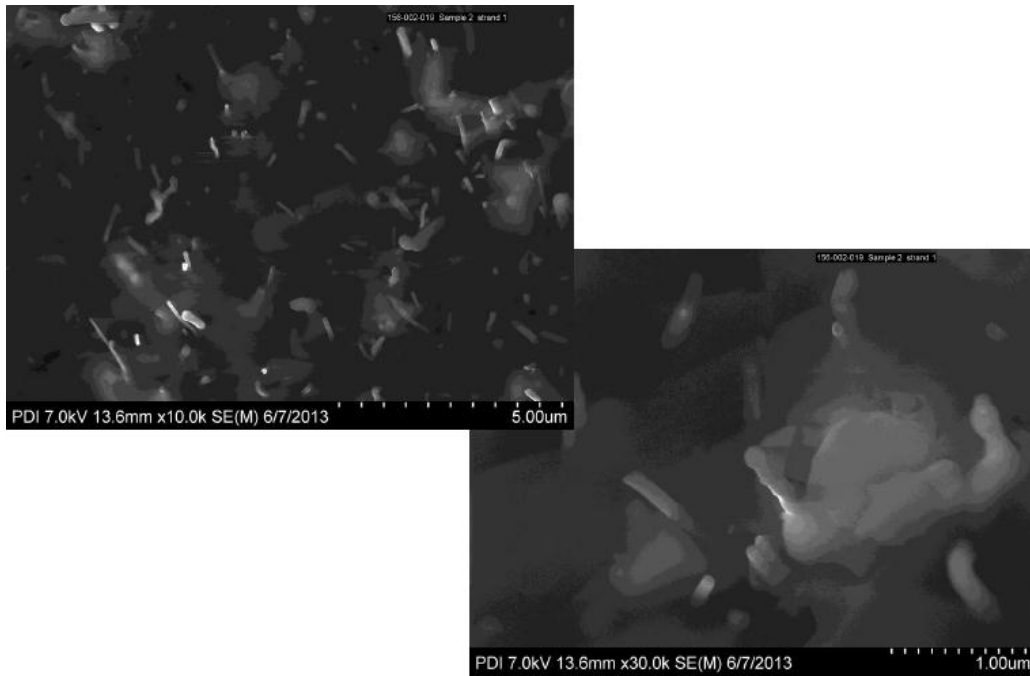
Figure 19.—SEM Characterization of uncured RTM370 with 10 wt% VGCNF.
