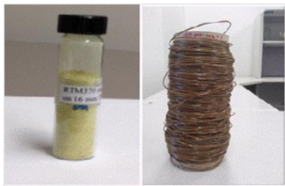
Figure 4.—Thermoset resin powder for use in Selective Laser Sintering (SLS) and thermoplastic filaments for Fused Deposition Modeling (FDM) types of 3D printers.
