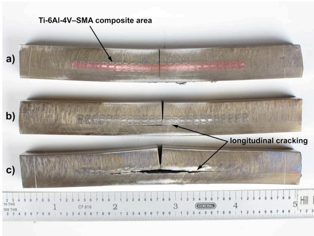
**Figure 4:** Side view photograph of as-tested cut compliance coupons: a) periodic mesh, cold rolled to 4% reduction, no memory activation heat treatment, b) periodic mesh, cold rolled to 4%, memory activation heat treatment, c) foam mesh, cold rolled 4%, memory activation heat treatment. For clarity, the Ti-6Al-4V-SMA composite area is highlighted by the red overlay in sample (a).
