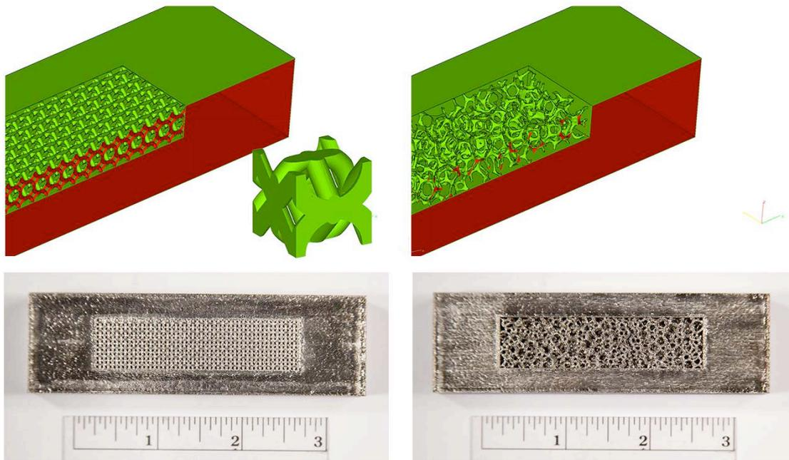
**Figure 1:** Test coupon designs (top) showing section cut through net structure area. Periodic design unit cell shown in inset, upper left. Actual as-fabricated test coupons made via electron beam melting shown on bottom.
