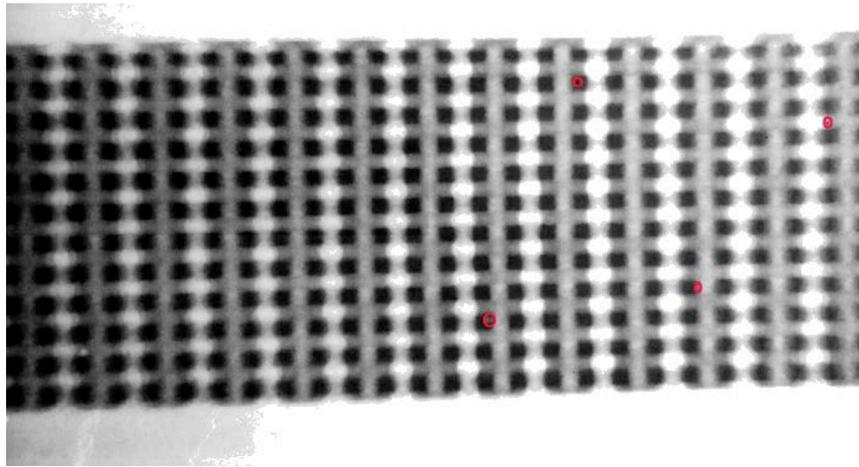
**Figure 2:** X-radiograph of as-consolidated periodic net shape structure. Red circles indicate isolated porosity.
