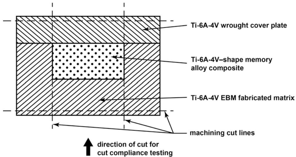
**Figure 3:** Schematic of the cross-section configuration of the coupons. The dashed lines show approximately how much material was machined away in order to prepare the coupons for cut compliance testing. Also note the arrow showing which direction the cut was made with respect to the coupon orientation.
