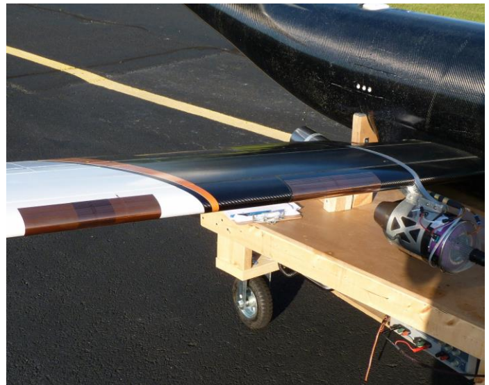
Figure 3. Close-up of the sensors at two span stations on the right wing
