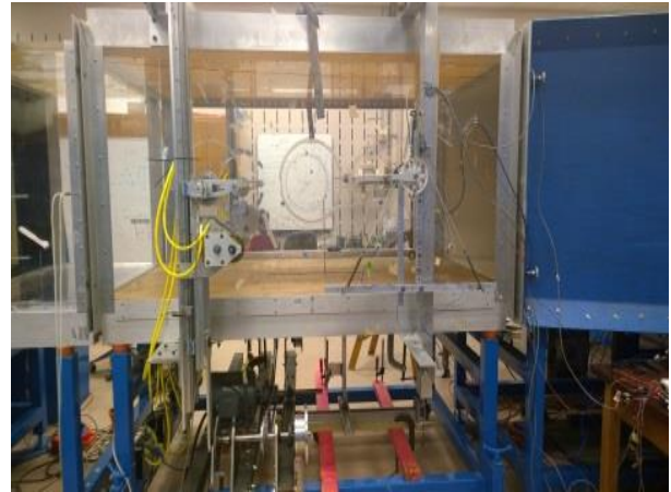
Figure 4: NATA II and PPDS (gust generator), flow direction from left to right
