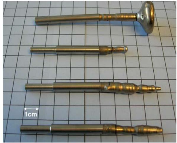
**Figure 2. Set of larger NiTiHf single crystals.**
