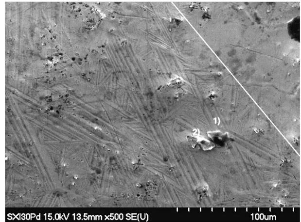
**Figure 3. SEM image of NASA grown NiTiPd single crystal at 500x. 1)TiC 2)W (Line marks edge of band)**
